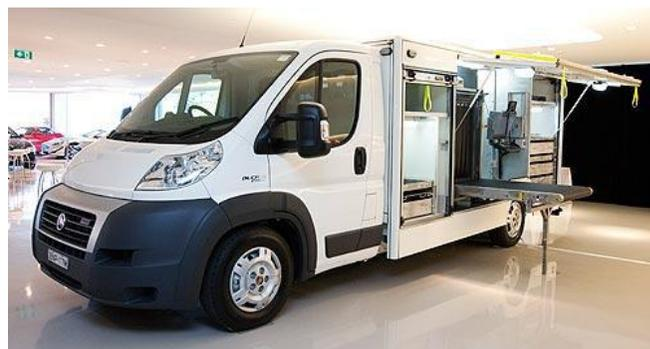
Emerging business trends indicated the need to increase the usage of the Mobile x-Ray units (MXUs) in the field. The MXU in operation at the time had usability issues causing staff injuries and risked damaging parcels, as well as placing unacceptable constraints on the composition of operator teams. Senior management appreciated the physical effort required to operate the MXU by performing the tasks themselves, which strengthened their support for the application of design thinking to new MXUs.
